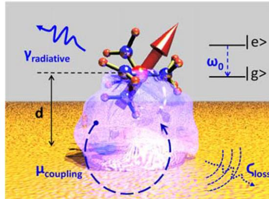
**Figure 1** Schematics of an open resonator – fluorescent molecule with a dipolar transition is coupled to a surface. Coupling mechanisms, coefficients and geometrical parameters are indicated on the figure.
