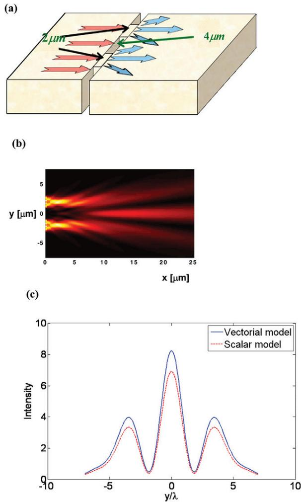
**Figure 6.** SPP Young's double-slit experiment. (a) Basic configuration. (b) Field intensity estimated by our full-vectorial model for comparison with experimental and theoretical data [17]. (c) Interference pattern at a distance of 15 wavelengths from the slits. Blue solid line, vectorial model; red dashed line, scalar model.
