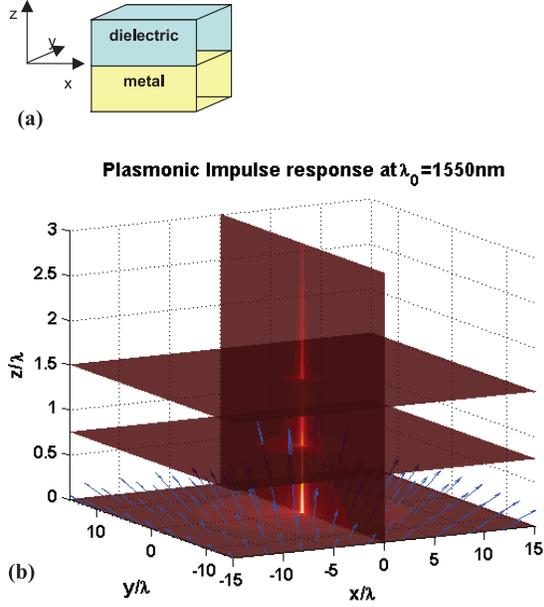
**Figure 1.** The SPP point source. (a) Dielectric/metal interface with coordinate system. (b) Electric field intensity of the SPP point source. The arrows indicate the polarization.
