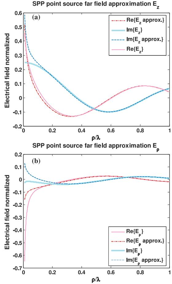
**Figure 2.** Electrical field of the SPP point source and its approximation by a cylindrical wave: (a) perpendicular (to surface) component; (b) parallel (to surface) component.
