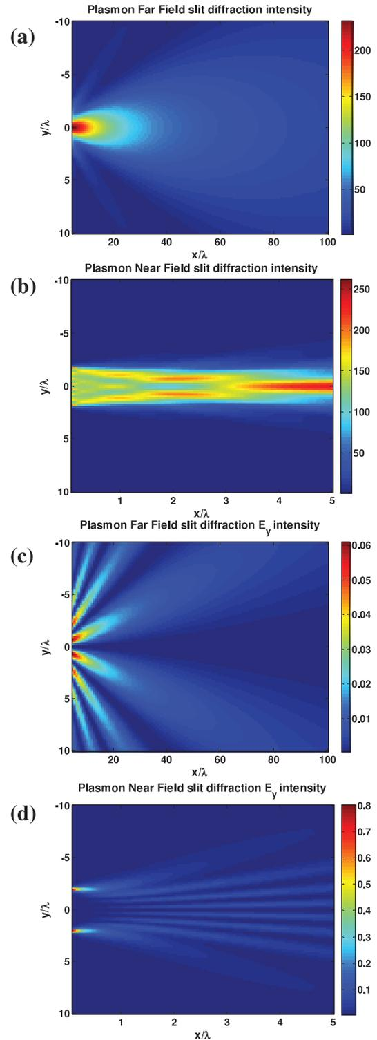
**Figure 3.** Single ( $4\lambda$ ) slit SPP diffraction pattern at  $1.55 \mu\text{m}$ . (a) Far field intensity. (b) Near field intensity. (c) Far field  $|E_y|^2$ . (d) Near field  $|E_y|^2$ .
