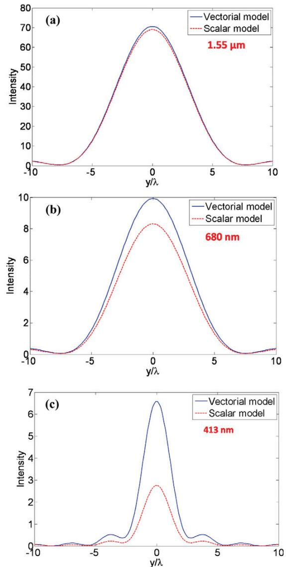
**Figure 5.** Single ( $4\lambda$ ) slit SPP diffraction pattern profile at a distance of  $30\lambda$  from the slit. Blue solid line, our vectorial model; red dashed line, scalar model. Excitation wavelength of: (a) 1.55  $\mu\text{m}$ , (b) 680 nm and (c) 413 nm.
