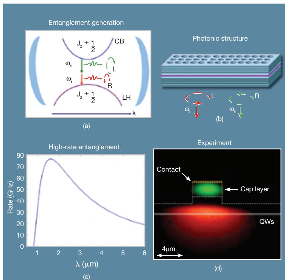
(a) Entanglement generation principle. (b) The proposed photonic micro-cavity structure. (c) The calculated emission rate vs. one of the TPE wavelengths in a cavity-controlled QW TPE entanglement source. (d) Experimental false color IR emission imaging of the facet of the QW-based waveguide. The upper lobe (green) is a parasitic 890 nm one-photon emission from the GaAs cap layer and the lower lobe (red) is the wide-band TPE from the QWs.
