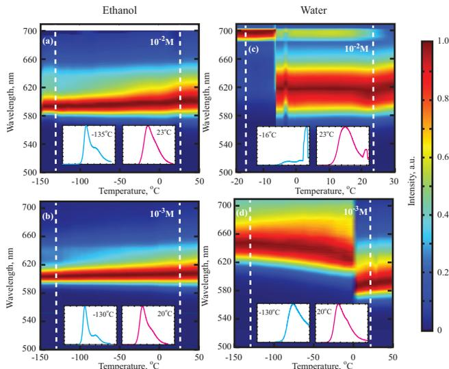
FIG. 1. Photoluminescence spectra of Rhodamine B solutions at different concentrations (rows) and solvents (columns). (a) ethanol,  $10^{-2}$ M concentration. (b) ethanol,  $10^{-3}$ M concentration (c) water,  $10^{-2}$ M, (d) water,  $10^{-3}$ M. All measured spectra were normalized to their maximum for each temperature point. Insets: slices of the spectra at the places, indicated with white dashed lines on the color maps.
